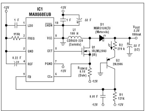
This PWM boost-controller IC provides relief to an overloaded 3.3V backplane supply by generating a supplemental 3.3V regulated output from the lightly loaded -12V rail of a VME, VXI, or PCI backplane.
